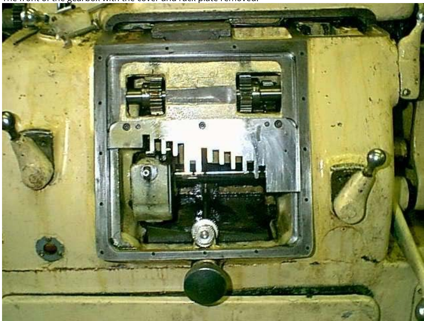
The rack plate with the tumbler attached on the right, and the backside of the front cover on the left.
