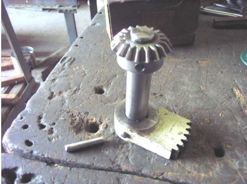
The nut block and 4 start worm. You can see the pin hole for attaching the worm to the reverse shaft. In this picture, the worm has already been shortened. The worm gives axial movement to the reverse shaft.
