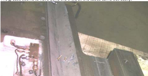
The Multifil hasn't been trimmed yet. I use a wood chisel, pushing against the CI base to trim. This is the V slide and you can see the 4 tubes sticking out of the oil holes. The last time I did this, on the CK in 2003, I didn't grease the tubes, and had a bit of trouble getting the tubes out. The grease seems to have done the trick, all the tubes came out easily.
