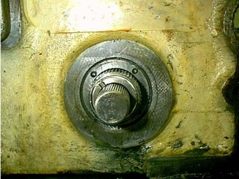
A better view of the leadscrew reverse mechanism, and for those of you who aren't familiar with this, I'm going to attempt to explain this. The large bevel gear is pinned to the shaft, which goes inside the headstock, and is pinned to the single dog clutch shifter yoke. Also pinned to this shaft is a three position detent, which is above the bevel gear. The small bevel gear is attached to the gear segment inside the gearbox, which meshes with the circular gear rack, which is pinned to the reverse rod, that runs the full length of the bed. The motion, left and right, of the rod, comes from the worm which inside the nut casting to the left. The rod's motion is imparted by the lever mounted on the apron; up, neutral, and down, which gives the feed direction.
