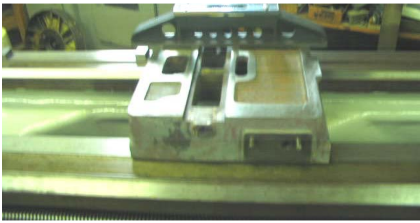
Checking the transverse way alignment. It's off a little, but I forgot how much.
