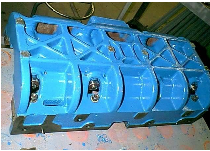
The shoe, swivel, slide TA draw rod, and gibs. The large holes in the gibs are for the eccentric studs.
