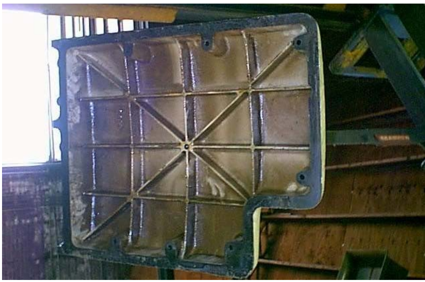
The inside of the headstock. It is 26" long approx. The bull has a 2" wide face, to give some perspective.
