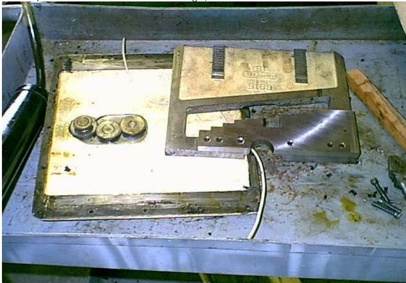
The rack plate with the tumbler attached on the right, and the backside of the front cover on the left.
