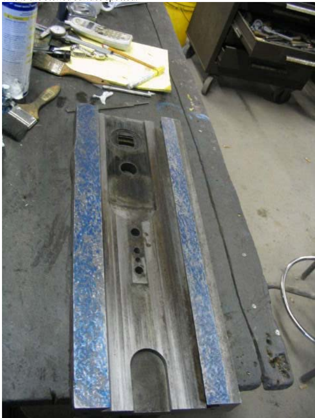
Same as above with the medium cleaned off. These are the surfaces I will use as a template to spot the cross slide ways.
