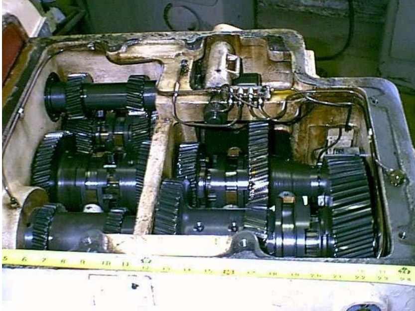
This is the clutch between the bull gear and the "Large and small spindle drive gear", with small one showing in the picture. It's hard to see but the corners of the clutch teeth are a bit chewed, probably from inadvertent shifts on the fly. I know I try avoid this, but every now and then it happens. The only potential problem I see here, is that this gear is used in the 8 highest speeds, and the load carrying capability may be affected.
