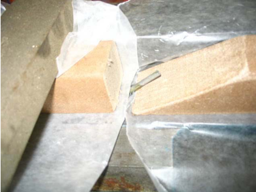
The Multifil hasn't been trimmed yet. I use a wood chisel, pushing against the CI base to trim. This is the V slide and you can see the 4 tubes sticking out of the oil holes. The last time I did this, on the CK in 2003, I didn't grease the tubes, and had a bit of trouble getting the tubes out. The grease seems to have done the trick, all the tubes came out easily.
