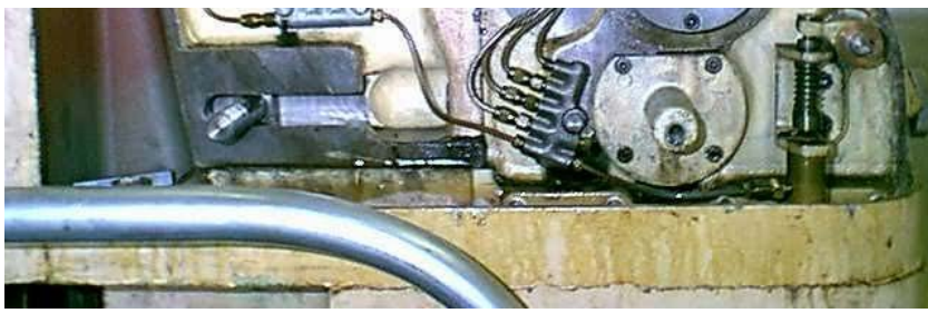
The 7th meter unit. To replace it, I would have to remove the shifter housing castings on the front of the headstock. It lubricates the right bearing of the C-D-E shaft.
