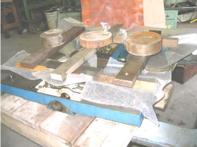
There are 3 sections of weights on each slide, here's the reason. I put lightly greased tubes in each of the oil holes to keep the epoxy out.
