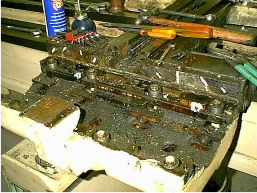
The slide, swivel and shoe came off as one unit.
