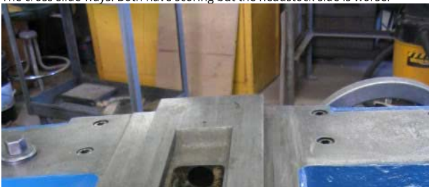
The cross slide ways. Both have scoring but the headstock side is worse.
