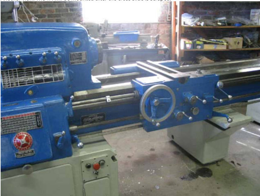
The cross slide ways. Both have scoring but the headstock side is worse.
