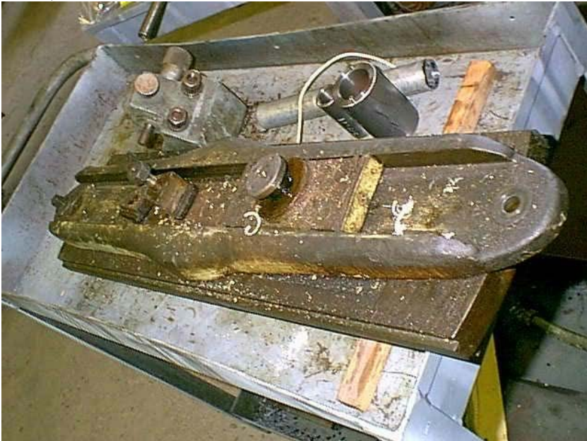
The cross feed screw and TA drawbar, compound rest and cross feed handle assembly.
