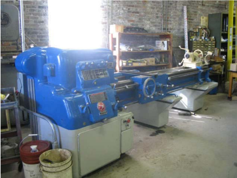
Another view. The TA will be mounted after the cross slide is scraped.
