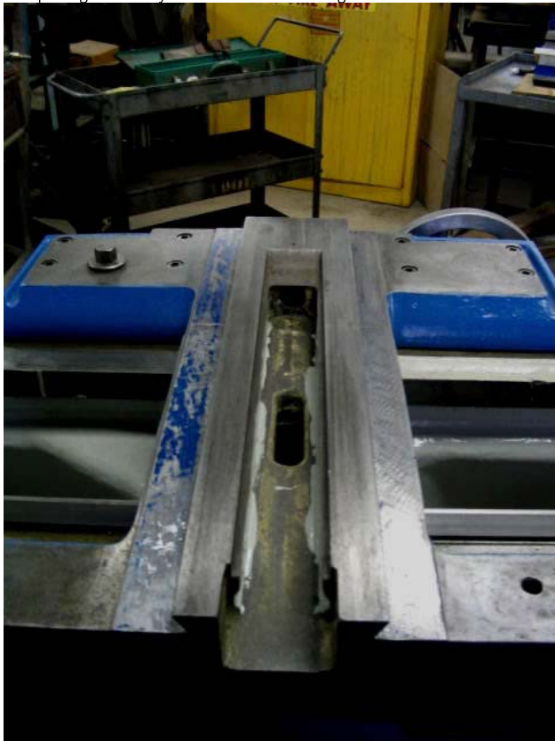
The picture is a little blurred, but this is how I get the cross slide on the ways to spot without cutting off fingers. It ain't easy.
