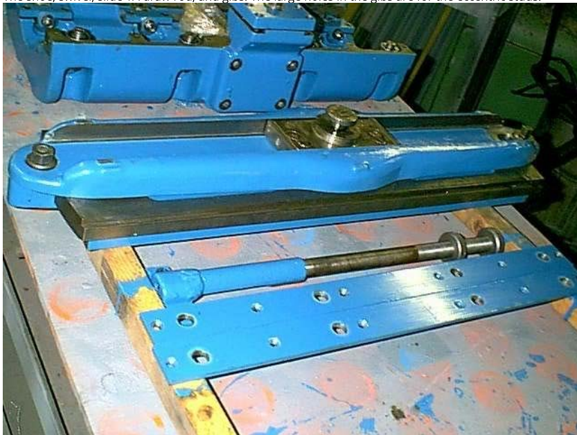
The shoe, swivel, slide TA draw rod, and gibs. The large holes in the gibs are for the eccentric studs.
