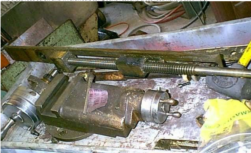
The cross feed screw and TA drawbar, compound rest and cross feed handle assembly.
