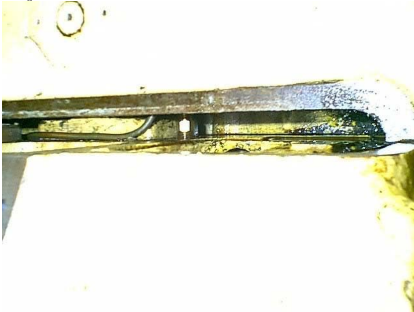
The front of the gearbox with the cover and rack plate removed.
