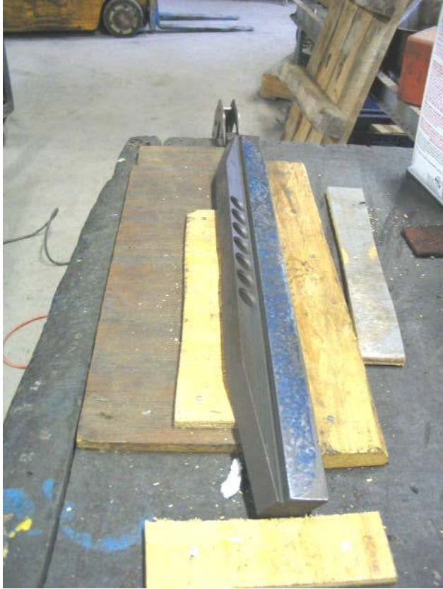
Surveying the cross slide ways. The ways were checked longitudinally and transversely. They are high in the right rear and low on the left front, the left side is lower than the right side. The objective is scrape the cross slide ways so that the level reads the same as it does for the bed, in both directions.
